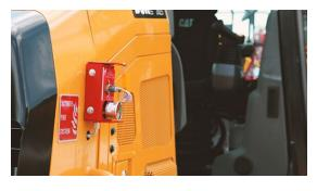
In the event of a fire, the Loss of Pressure (LOP) is detected through the pressure tubing automatically activating the system to dispense the Fluorine Free Foam from strategically placed nozzles to extinguish the fire. The fire alarm panel is also triggered which alerts the operator and surrounding personnel of the situation. The shutdown panel (when fitted) will further shutdown the engine after predetermined times to prevent the continued fuel supply to the fire.
