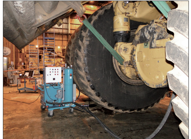
The CJC™ Mobile Flushing Unit, MFU looks small while performing a hot-flush of the 797 differential
