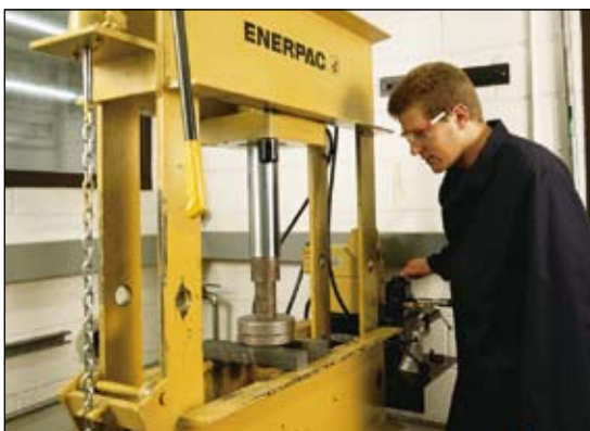
◀ An Enerpac H-Frame press makes quick work of removing the shaft from this assembly.
