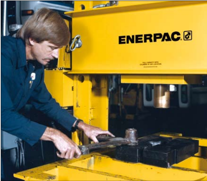
▲ An IPR-20075 Roll-Frame Press is used to remove a large shaft from this pillow-block assembly. The Roll Frame design allows this heavy part to be safely loaded with an overhead crane.
